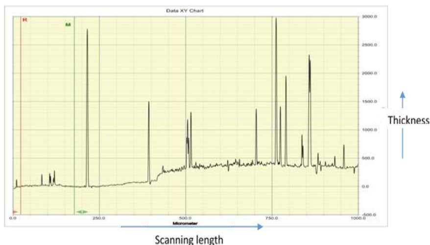
Figure 9: A line Profile for \text{TiO}_2 sprayed with 0.3ml for 3minutes at substrate temperature of 400^\circ\text{C}
