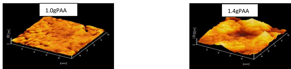
Figure 5: AFM images for CZTS thin film samples
