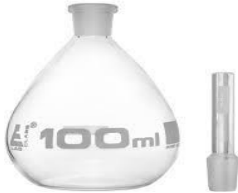
Figure 6: Photograph of a calibrated pycnometer used in the determination of specific gravity
