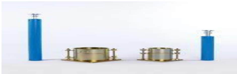
Figure 9: Photograph showing mold and rammer used for compaction test
