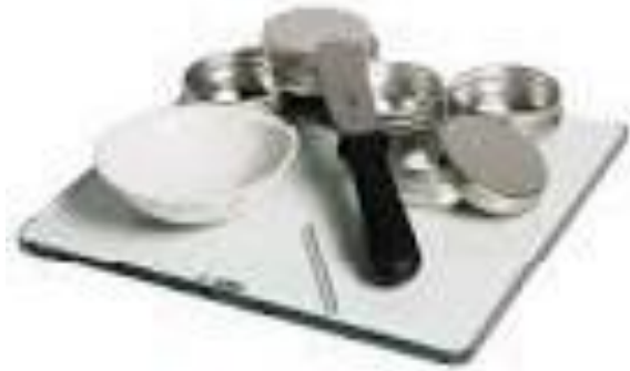
Figure 7: Apparatus for Plastic limit test
