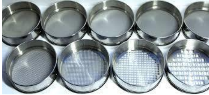
Figure 5: Photograph showing the set of sieves used for the determination of coarse grain analysis
