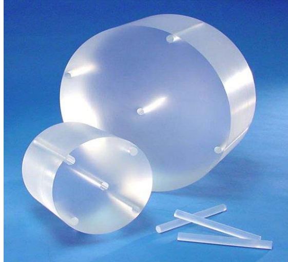
Figure 2: The 16 cm and 32 cm cylindrical CTDI phantom with the acrylic plug or rods to be inserted at the five holes within the phantom
