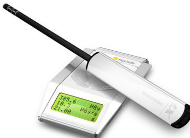
Figure 1: UNFORS RaySafe Xi CT dosimeter for CTDI measurement used in this study
