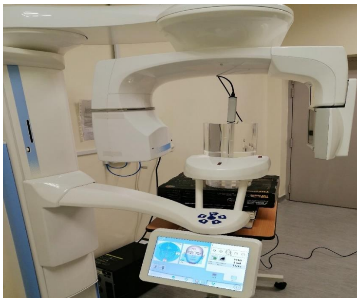
Figure 3: The CTDI phantom sized 16 cm with the UNFORS CT dosimeter were positioned on the CBCT holder during the dose measurement
