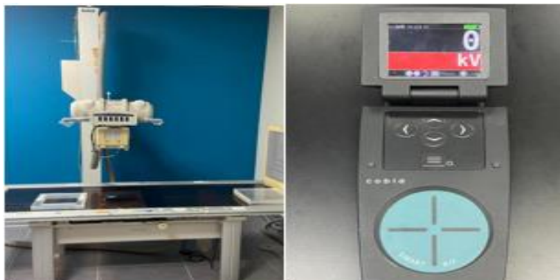
Figure 1: (a) X-ray Machine for Exposure and (b) Ionization chamber dosimeter (Cobra)
