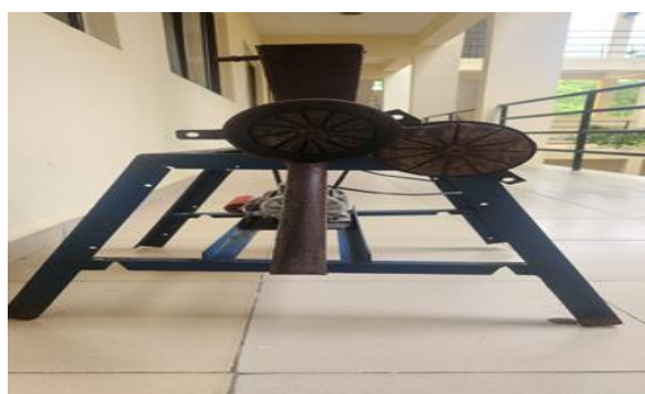
Figure 1: Design views showing the feed hopper, shaft and beater-conveyor assembly
