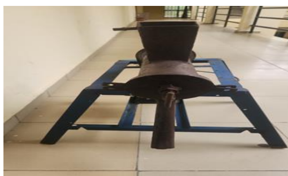
Figure 1: Design views showing the feed hopper, shaft and beater-conveyor assembly
